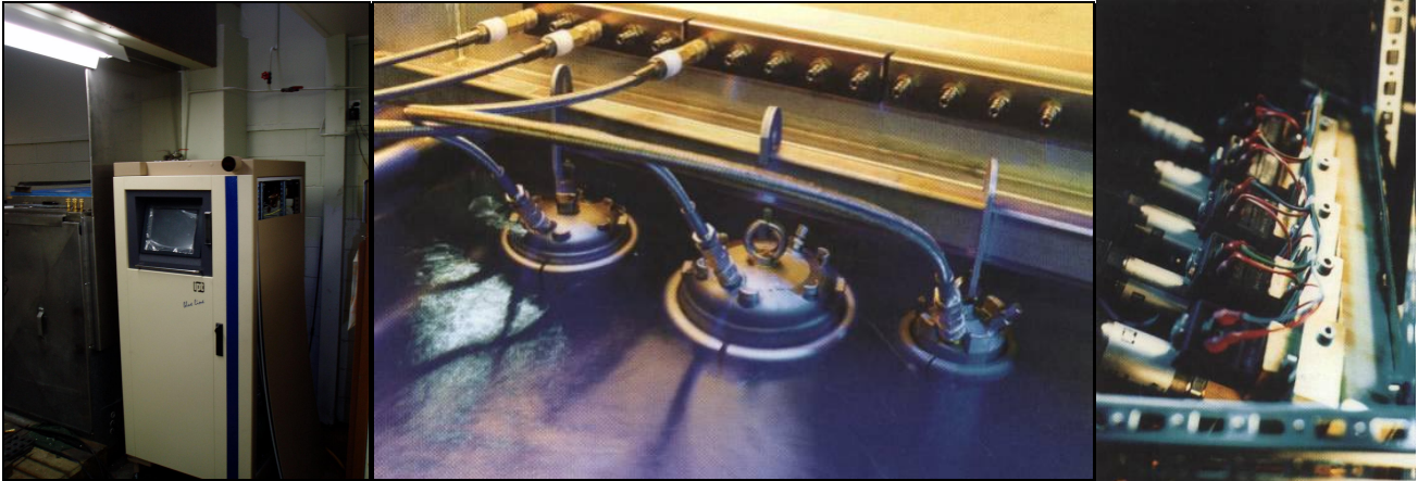
The IPT BlueLine Series accommodates up to 20 individual samples to your nominated pressure range
